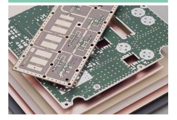
RT/duroid<sup>®</sup> 5870 and 5880 glass microfiber reinforced PTFE composites are designed for exacting stripline and microstrip circuit applications.
